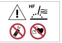
As welding by the TIG method or plasma cutting involves high frequency ignition, it can interfere with mobile phones, radio equipment, TV equipment or improperly protected computers and industrial robots, which leads to total disabling of such devices.
