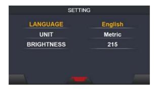
Press the functional parameter button (D) and hold it for 3s to enter the system interface. Here you can adjust the language, the unit and the brightness setting by left and right welding adjustment knob.
