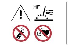
As welding by the TIG method or plasma cutting involves high frequency ignition, it can interfere with mobile phones, radio equipment, TV equipment or improperly protected computers and industrial robots, which leads to total disabling of such devices.
