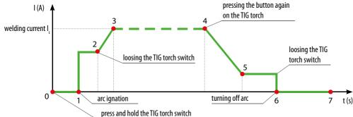
0 Press and hold the gun switch, Electromagnetic gas valve is turned on.
