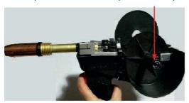
**10.** Feed the wire through the drive rolls and into the inlet guide tube. Tighten the wire tension swing arm.
