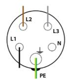
L1, L2, L3 Phase conductors
