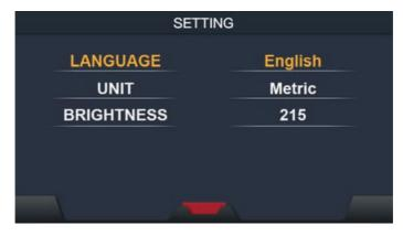
Press the functional parameter button  $(\mathbf{D})$  and hold it for 3s to enter the system interface. Here you can adjust the language, the unit and the brightness setting by left and right welding adjustment knob.
