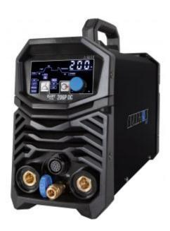
The SPARTUS® EasyTIG 206P DC is a technologically advanced inverter welder based on IGBT transistors and PWM technology. It offers TIG HF/LIFT and MMA welding methods with amperage up to 200A, powered by a single-phase 230V network.
