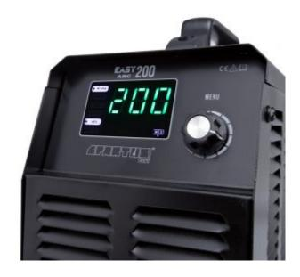
The EasyARC 200 is powered by a single-phase 230V power supply, which means it can be used in various locations, both in workshops and on-site. The welding current can be adjusted within the range of 30 to 200A, providing flexible adaptation to diverse welding tasks. The device has sufficient power for welding coated electrodes up to 5.0mm in diameter.
