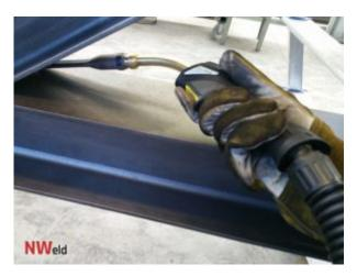
Construction and shape of gas nozzle allows to weld with good observation of welded joint and minimum adhesion of spatter without need to use of antispatter liquid spray.
