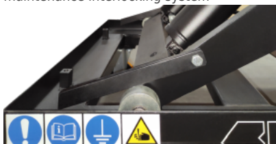
maintenance interlocking system
