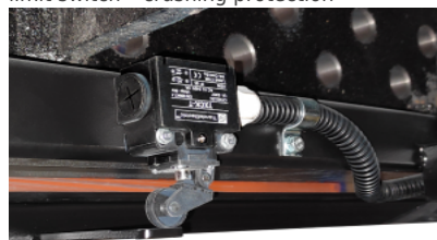
limit switch – crushing protection
