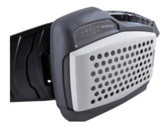
The SPARTUS® air supply system has a high level of respiratory protection TH3P thanks to a set of replaceable filters, including a main HEPA filter and an activated carbon pre-filter. The whole system is protected by a spark shield. The connection between the breathing hose and the visor housing provides freedom of movement during work.
